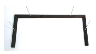
Step 4: Insert 100 mm wooden part for gaps (C) through each threaded rods (D).
