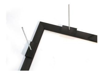
Step 5: Insert another frame through the threaded rods. Repeat steps 4 and 5 in turns as long as you reach the seventh frame.
