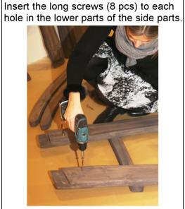
Adjust the crossbars between side parts, tighten the screws.
